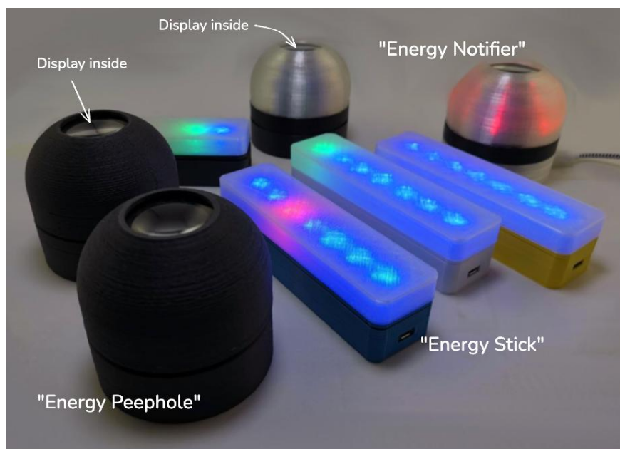
Figure 3.2: The Energy Inspector devices (RPI): Energy Peephole, Energy Stick, and Energy Notifier
