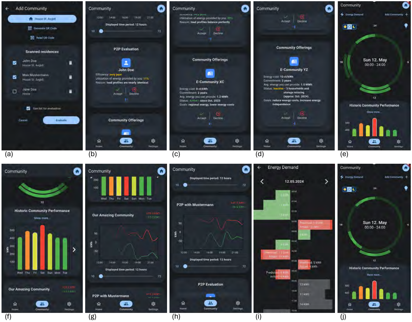
Fig. 2. Screenshots of the end-user mobile application for facilitating EC and P2P energy trading. (a) Interface for generating and scanning QR codes to form an energy community. (b) Results of the feasibility studies for P2P. (c) Details of an offer from functional EC for the user. (d) Identification of a planned EC. (e) Visual overview of personal demands vis-a-vis EC demands. (f) Historical EC performance of a week. (g) Monitoring of EC performance based on near real-time data. (h) Performance of P2P energy sharing based on near real-time data. (i) Interface for predicting demand and surplus energy by end-users and monitoring the accuracy of their predictions. (j) Example of the relation of the user with another EC where the symbiotic relation is more prominent.
